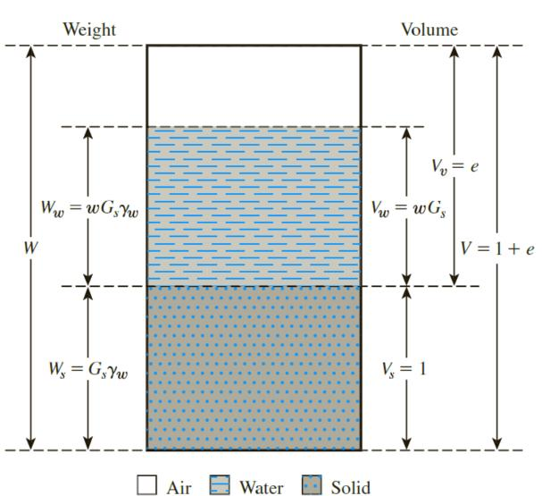
• Relationships among Unit Weight, Void Ratio, Moisture Content, and Specific Gravity (saturated Case)
